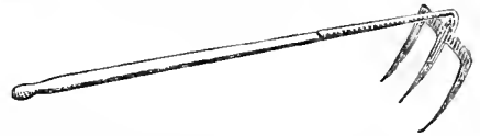
No. 1.—Length of handle, including iron socket, 4 feet 9 inches; diameter of handle, 1½ inch; width of the head, 6½ inches; length of curved teeth, or prongs, 6¼ inches.
